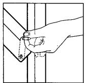
included with your range, into both hinge hangers. **Do not** remove the pins while the door is removed from the range.
